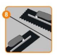
The bigger the size of tile, bigger is the notch of the trowel (from1/4"to1/2") and lesser is the coverage (4 to 8 sq.Mt.) Per 30 kg. Bag.
