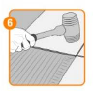
Tap the tiles gently with a wooden hammer after laying for proper fixing/leveling.
