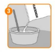
Mix WONDERFIX and clean water in the ratio of 5:1 by volume. Pour water in a container and add WONDERFIX slowly along with continuous stirring and mixing and prepare a consistent and thick mix.
